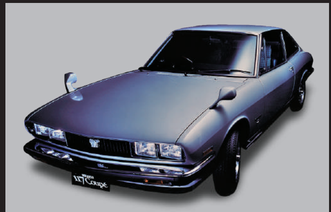
The late model underwent significant revisions to both the interior and exterior. The headlights changed from round to rectangular, and a chin spoiler was added. To facilitate mass production, the interior was simplified.
