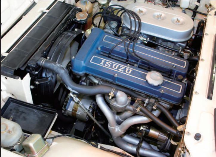
The G161W engine, Isuzu's first DOHC engine, was developed specifically for the 117 Coupe. Initially, only the 1600cc variant was available, but it was standardized to 1800cc following a minor change in 1973.
