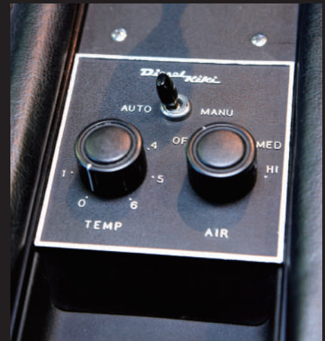
The cooler switch was in front of the shift lever on the center console. This layout was also typical of European cars at the time.
